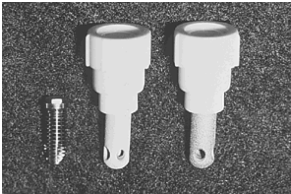
Fig. 2 Test implants with three different surfaces, shown left to right: titanium alloy (Ti-A), hydroxyapatite-coated (HA), and titanium plasma-sprayed (TPS).
