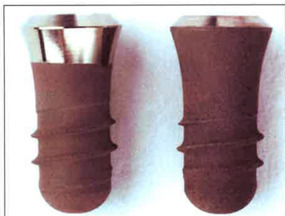
Fig 3 (Left) The most coronal 1.8 mm of the control implants (left) had a relatively smooth machined titanium surface; the remainder of the 9-mm implant had an SLA surface. The test implants (right) had no machined collar; thus, the SLA surface was 9 mm in vertical height.
